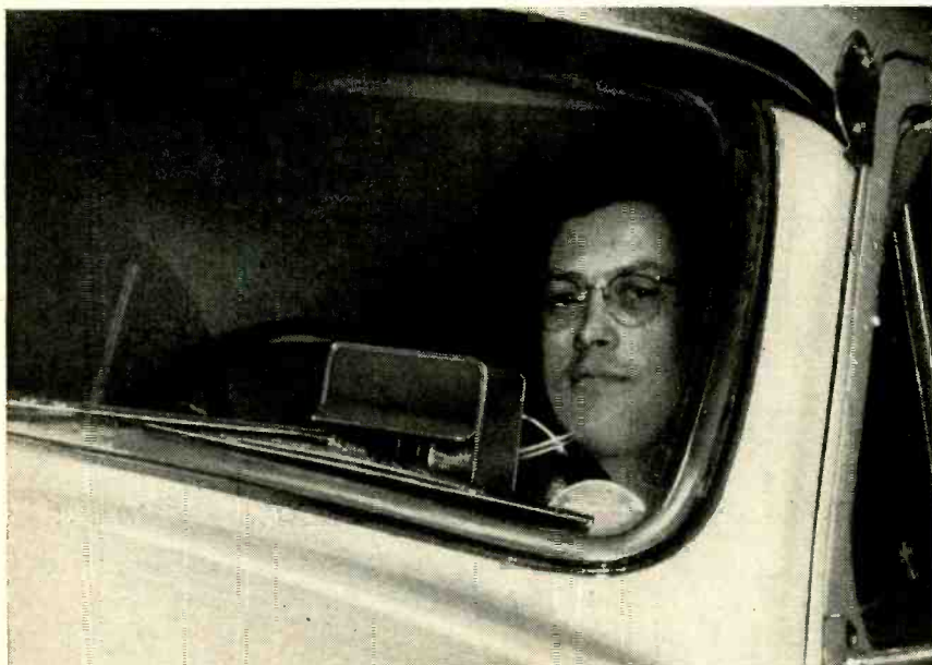
Electronic headlight dimmer installed. Oncoming headlights actuate dimmer.
